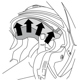
4. Connect the 2 pins of the back pad with the plug-in devices. Press the open end over back pin of the cheek pad.
