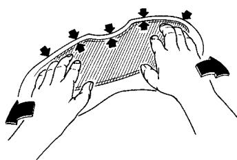
5. Ensure that the anti-fog lens sits snugly on the visor. If this is not the case, the tension on the anti-fog lens can be increased or decreased, as necessary, by turning the eccentric holding pin.
