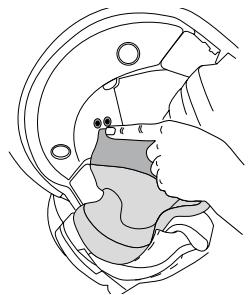
3. Fasten the forehead pad to the 4 holders and connect the pins with the corresponding plug-in devices.
