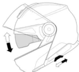
The maximum opening position of the sun visor can be set using the limiter. The limiter is on the running edge of the sun visor slider.
