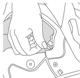
4. Press the retaining element inwards out of the sun visor. Repeat this step on the other side.
