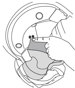
4. Loosen the 2 pins of the back pad.
